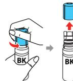
Caution : Do not shake or squeeze the ink bottles. Do not touch the top of the ink bottle after its cap is removed.
