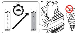
Note : Ink flows into the tank and stops automatically when the ink is filled to the upper line. If ink does not flow from the bottle, lift and reinsert the bottle.
