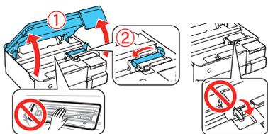
Caution : Do not touch the areas shown inside the product. The printer ships with the transportation lock in the printing position. Do not move it from the printing position.
